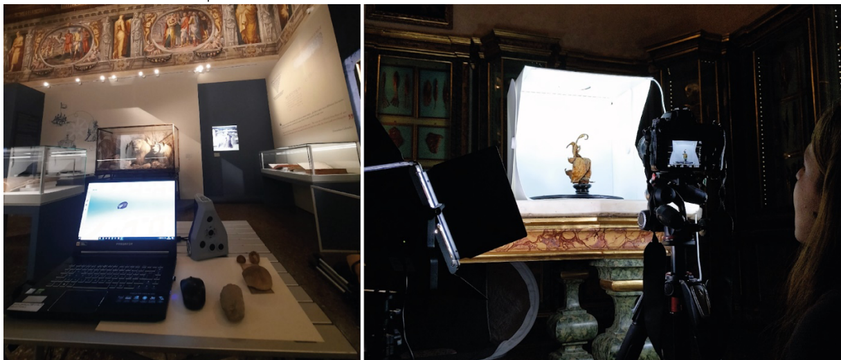
Researchers acquiring different types of objects using a structured light projection scanner (left) and photogrammetric techniques (right) and using supports such as a camping table (left) and a marble table (right)
